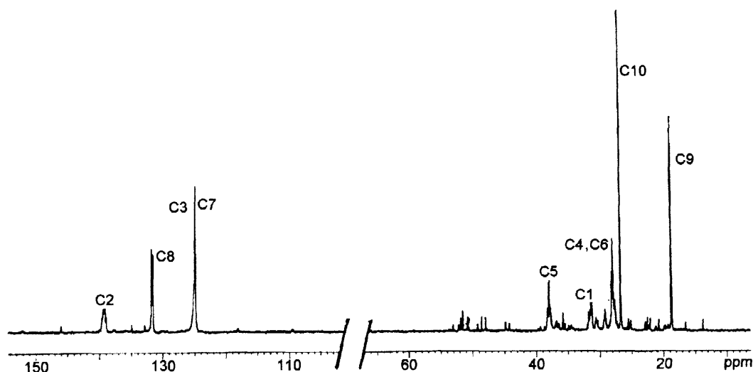
Figure 4. ^{13}\text{C} -NMR spectrum ( \text{C}_2\text{D}_2\text{Cl}_4 ) of the polymer fraction of gum mastic.
